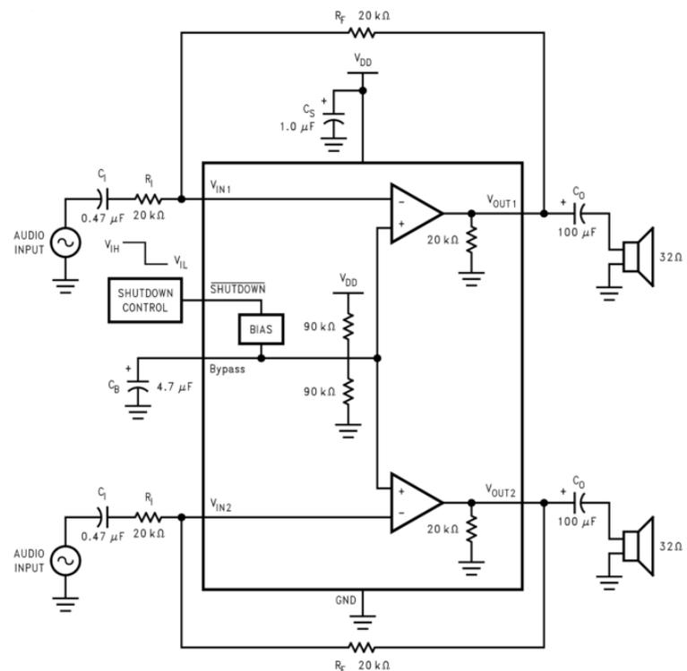
Figure 1. Application Circuit
